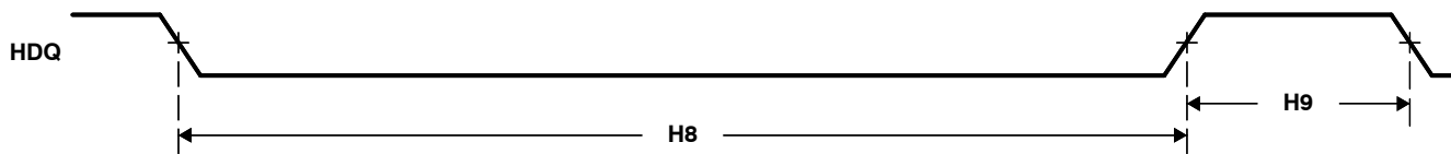
Figure 5–39. HDQ/1-Wire Break (Reset) Timing
